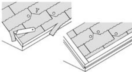
Figure 10-19: Preparing an old roof for reroofing.
