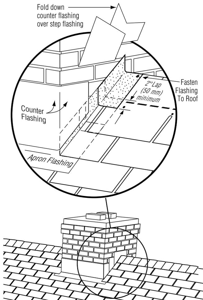
*Figure 10-18: Flashing around a chimney.*
